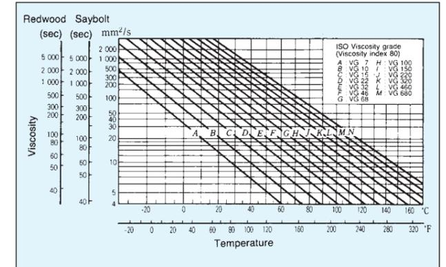
**Fig. 4.1** Relation between oil viscosity and temperature
